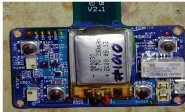
Figure 1: Top of the PoNS™ Neuro-stimulator board
