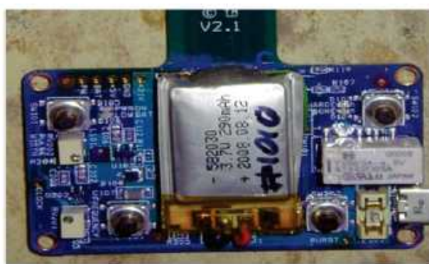
Figure 1: Top of the PoNS™ Neuro-stimulator board
